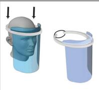
Place headgear over the crown of your head. Position to a comfortable fit. To tighten; secure the back ends with a rubber band, hair tie or zip tie.
