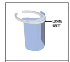
Slide the shield down until the hole locks into place.
