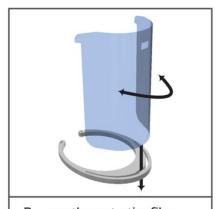
Remove the protective film from the PETG / Polycarbonate shield. Bend the shield and slide it into the top curved slot of the headgear.
